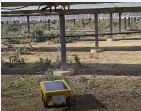
Autonomous robot tests for vegetation clearing in photovoltaic plants
