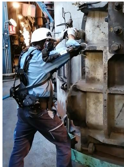
EXOSKELETON: Validation tests for the use of exoskeleton to reduce physical effort in field activities
